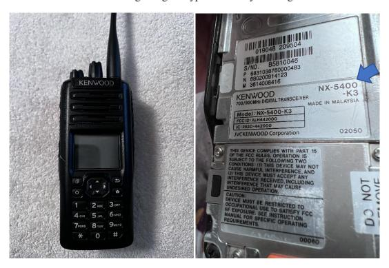
As it is seen in the picture above the model number beginning with the NX characters indicates that this model is to be replaced, so any agency using this modl please be aware of the need for replacement by July 1<sup>st</sup>, 2025.
